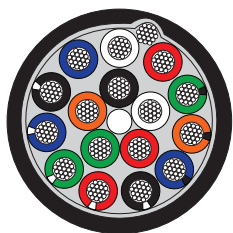
Type: P16C16# OS 16 conductors, 16 AWG Overall screen with foil and drain wire Nominal cable OD: 0.560", 14.23 mm
