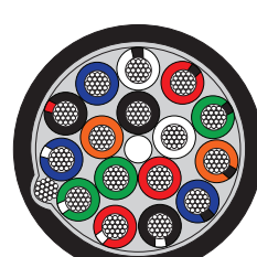
Type: P16C20# OS 16 conductors, 20 AWG Overall screen with foil and drain wire Nominal cable OD: 0.409", 10.40 mm
